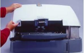
5. Remove the separator module by pulling it down and lifting it off.
